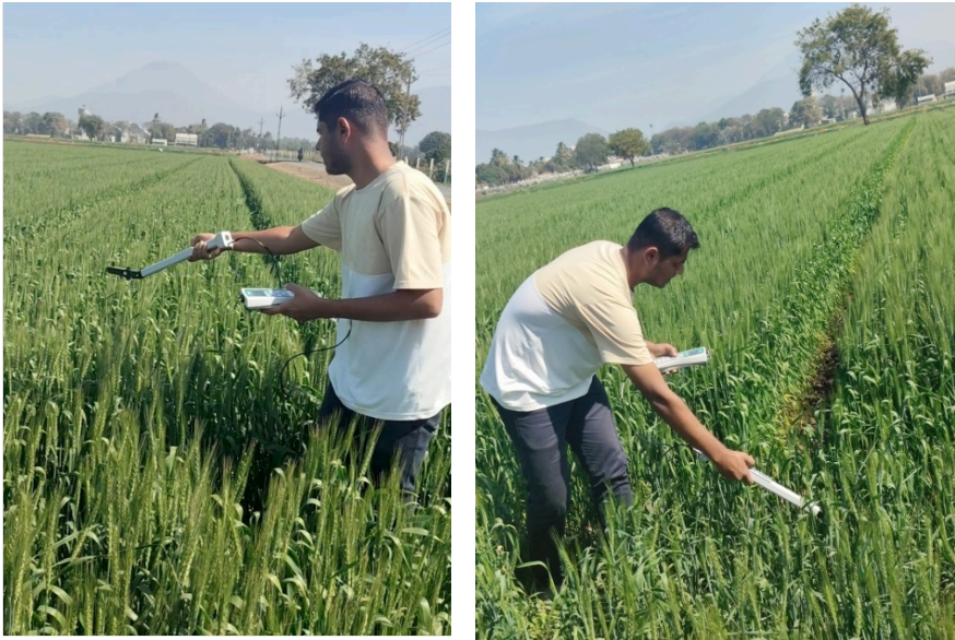
Figure 1. In-field measurement of Leaf Area Index (LAI) using the LAI-2200 Canopy Analyzer, above (A) and below (B) the canopy
