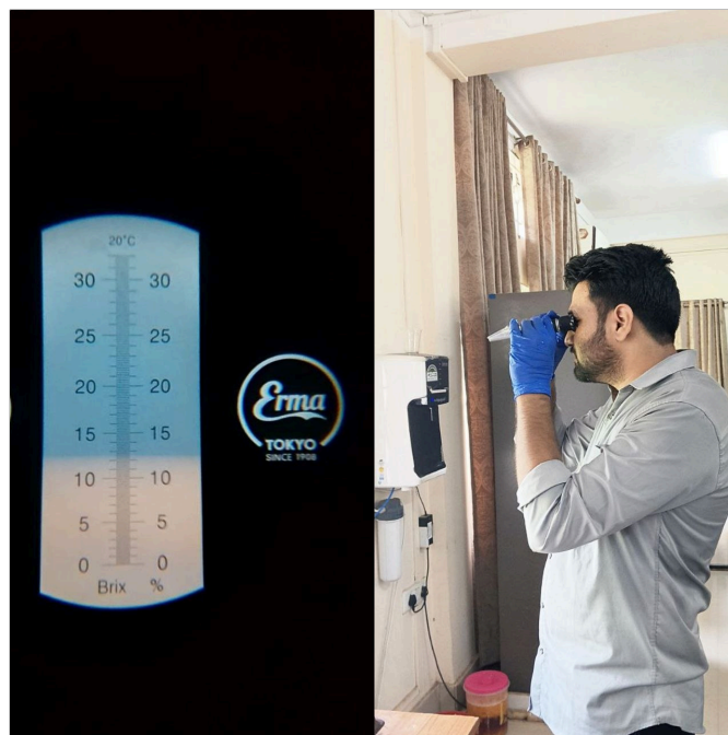
Figure 2. Measurement of total soluble solids (TSS) using a hand refractometer
