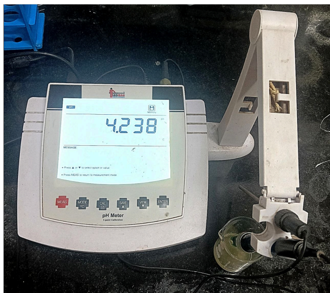
Figure 3. Measurement of juice pH using a calibrated digital pH meter
