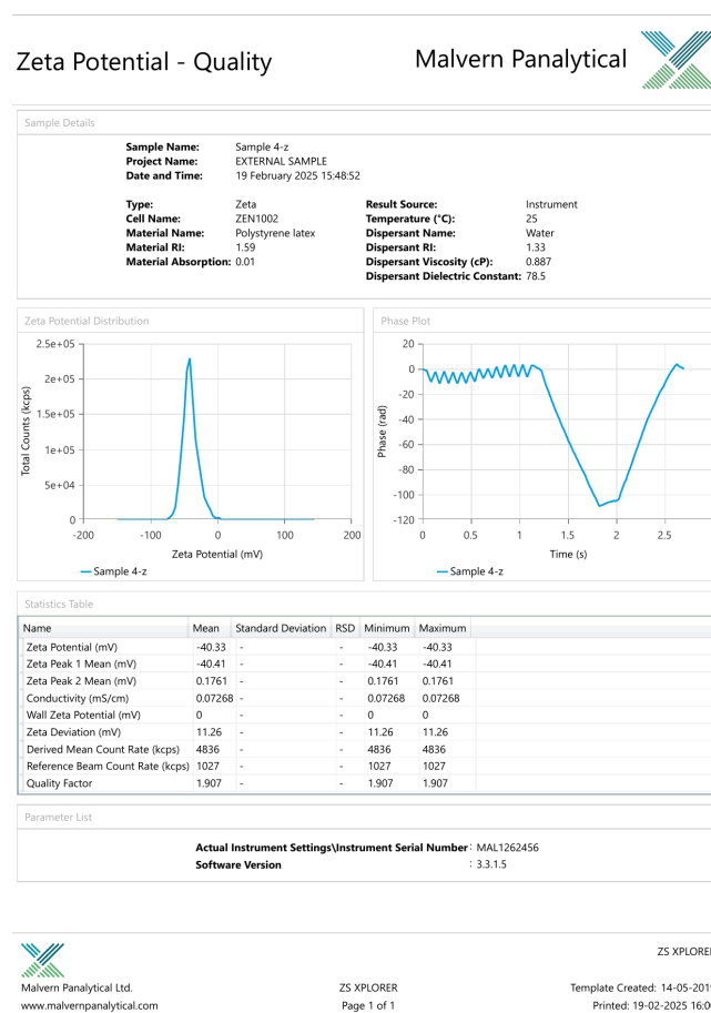
Figure 6. Malvern Panalytical zeta-potential report for the NanoCal Se sample, showing a mean zeta potential of -40.33 mV and principal peak mean of -40.41 mV.
