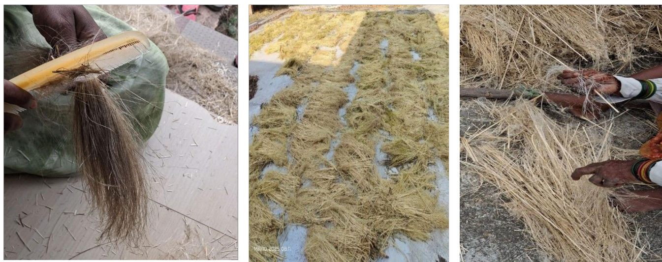
Figure 3. Sun Dried, Scutching and Hackling of Flax Fiber
