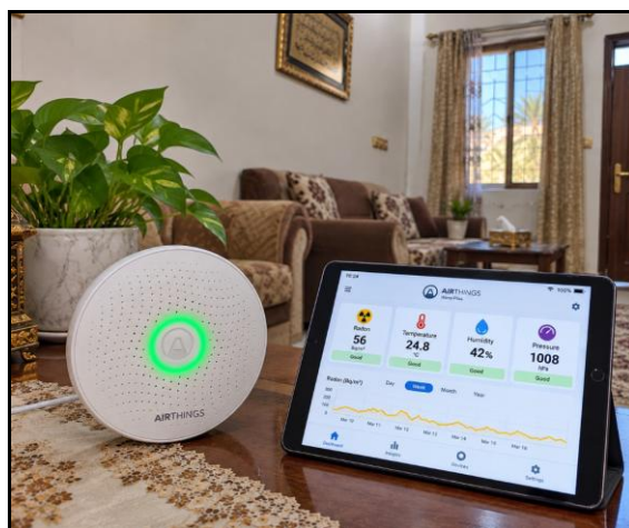
Fig 2: Airthings Wave Plus (Model 2930) used for measuring indoor radon concentration and temperature in the selected residential houses of Maytham Al-Tammar District, Al-Kufa City.
