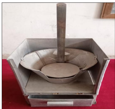
Plate 2.2: Measurement of angle of repose of groundnut pod
