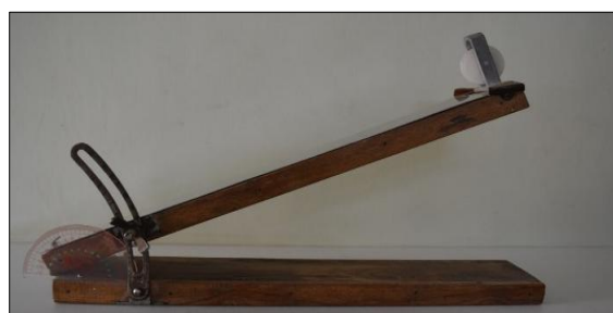
Plate 2.3: Experimental setup for measurement of coefficient of friction
