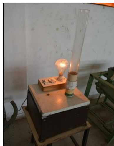
Plate 2.4: Experimental setup of air column for determination of terminal velocity
