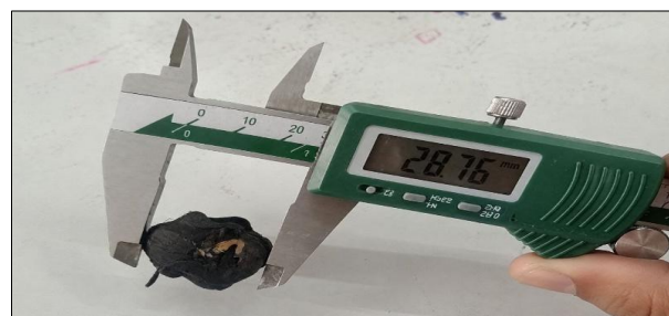
Plate 2.1: Measurement of water chestnut thickness using vernier calliper
