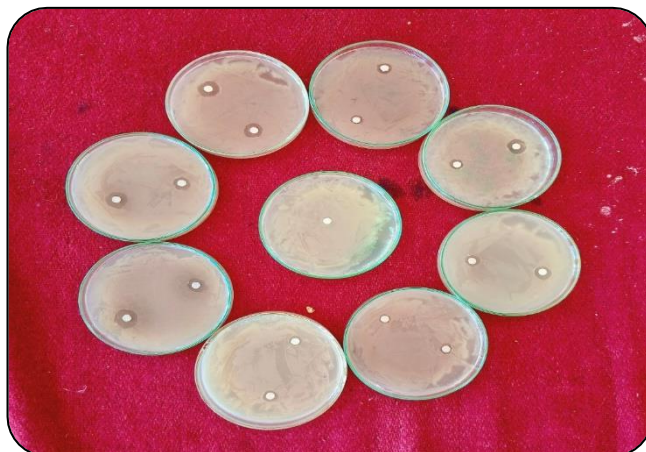
Note: In each Petri plate, the inner paper disc represents the lower concentration (1%), whereas the outer paper disc represents the higher concentration (2%) of the respective chemical.
