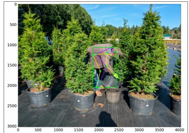
Fig 8: Output of MoveNet for Human Posture Estimation
