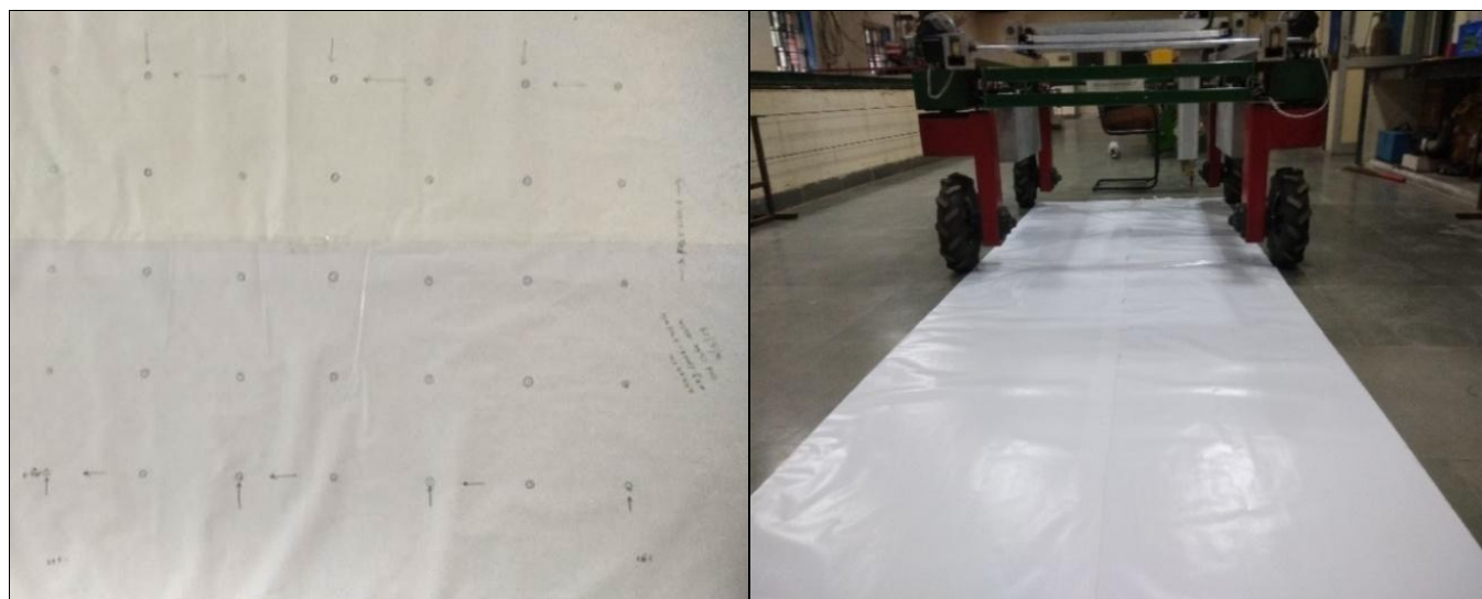
Fig.3: (a) Laboratory testing setup using graph paper (b) Marking done by the robot on paper
