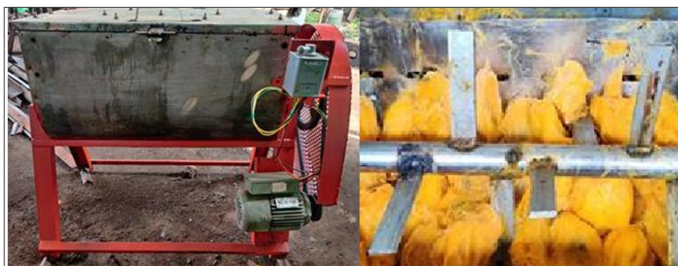
Fig 2: Palmyrah fruit pulp extractor with inside view (Vengaiah et al. ., 2023) [22]
