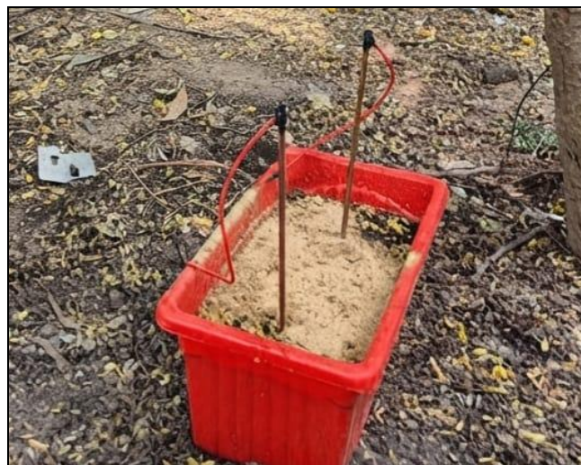
Fig 1A: Experimental setup before sowing showing the low-voltage DC electroculture system. Two copper electrodes connected to a 9 V battery were inserted into opposite ends of the pot to provide continuous electrical stimulation
