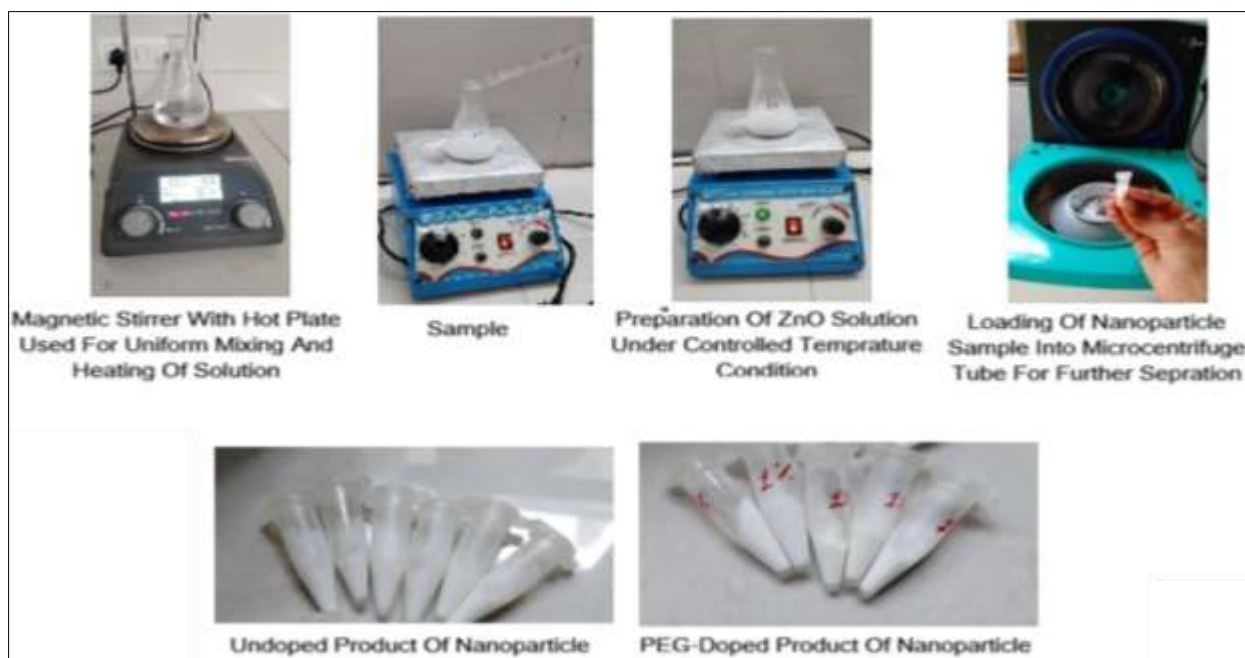
Fig 1: Schematic diagram of experimental setup for synthesis of undoped and peg-doped ZnO nanoparticles
