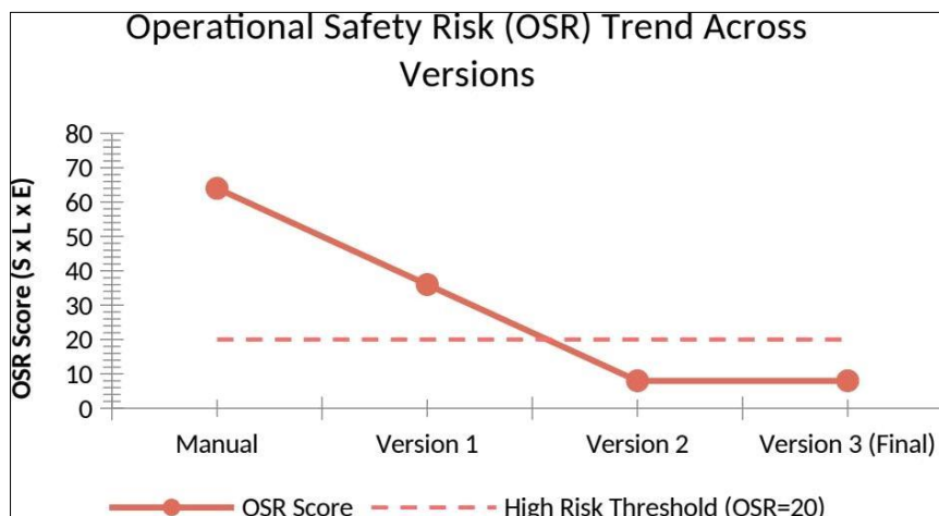
Fig 9: OSR score trend across design versions. The dashed red line marks the High Risk threshold (OSR = 20). Manual operation and Version 1 fall in the High Risk zone; Versions 2 and 3 achieve Low Risk status (OSR = 8)
