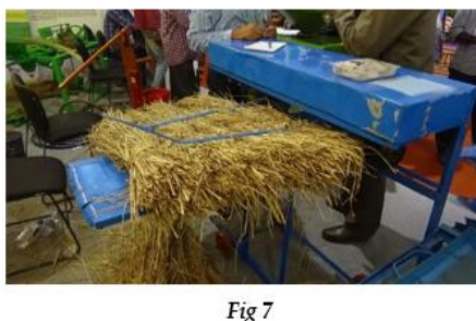
Fig 5, Fig 6, and Fig 7 collectively showing Third and final version of the straw cutter having improved feeding tray, guiding bars, and motor assembly
