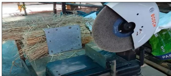
Fig 3: First version of the straw cutter (single-blade motor-operated)
