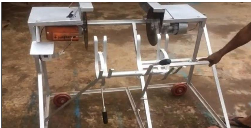
Fig 4: Second version of the straw cutter with manual feeding tray and safety housing
