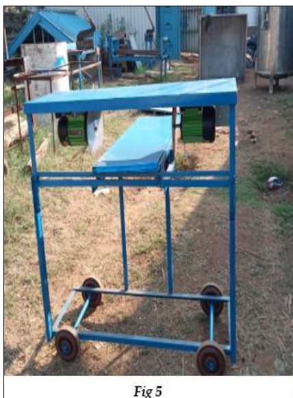
Fig 5, Fig 6, and Fig 7 collectively showing Third and final version of the straw cutter having improved feeding tray, guiding bars, and motor assembly
