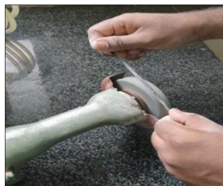
Fig 3: Preparation of horn peg on grinding machine
