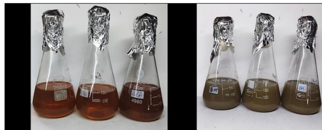
Fig 1: Biosynthesis of AgNPs using secondary metabolites of S. diastaticus (a) reddish appearance of supernatant of S. diastaticus before the addition of \text{AgNO}_3 solution (b) reaction mixture of cell-free supernatant and \text{AgNO}_3 solution showing a dark olive-brown colour after 24 h of incubation, indicating AgNPs formation.
