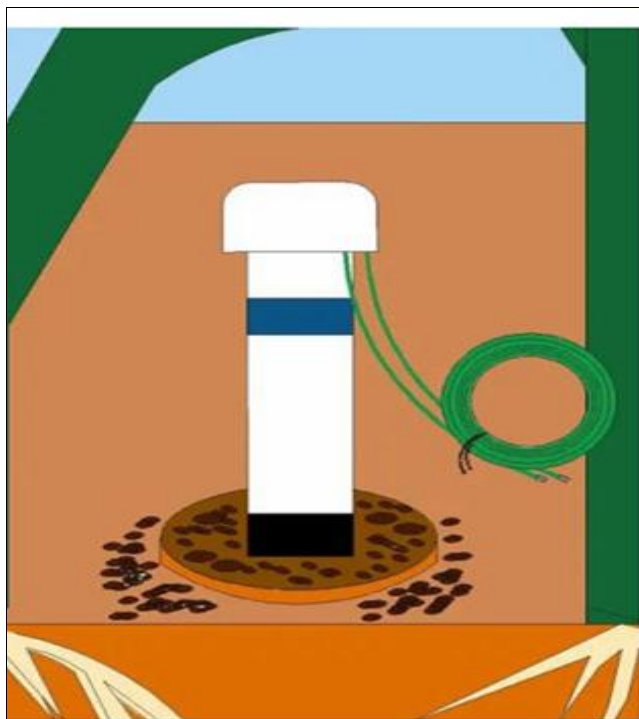
Fig 4 (c): Installed electrical resistance soil moisture sensor in the field
