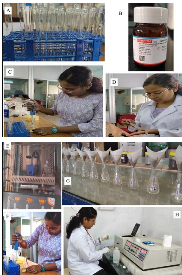
A: Airtight screw cap test tube B: TTC C: Adding of TTC to the sample D: Mixing of sample with TTC E: Incubation F: Adding ethanol after incubation G: Filtration of sample H: Reading on spectrophotometer
