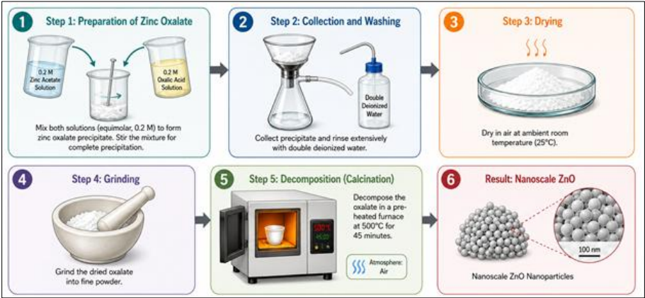
Fig 1: Synthesis of nanoscale ZnO by oxalate decomposition technique
