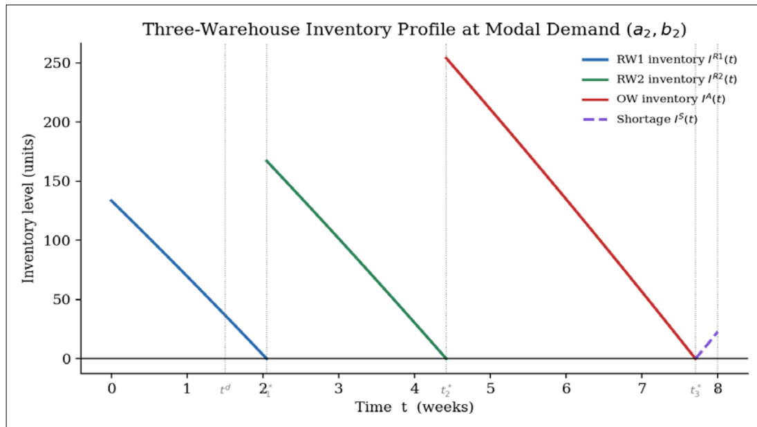
Fig 1: Three-warehouse inventory profile at modal demand ( t_1^*=2.05 , t_2^*=4.42 , t_3^*=7.71 weeks)
