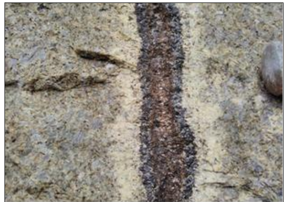
Fig 8: Phlogopite vein at syenite-pyroxenite contact
