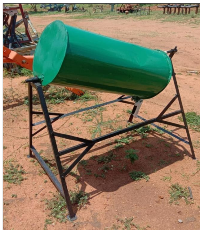
Fig 1: Model of the seed treatment drum simulated
