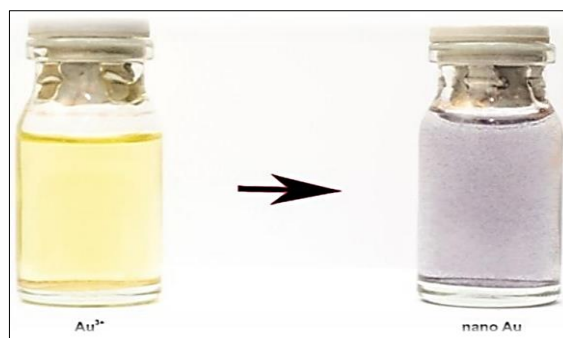
Fig 2: The gold solution color change from yellow to purple after adding glucose and PVP
