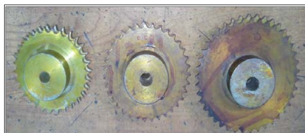
Fig 2: 30, 35 and 40 number of gear teeth for pigeonpea metering
