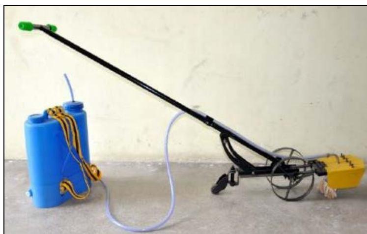
Fig 28: CRIJAF Herbicide Applicator for non-selective herbicide application in field and horticultural crops for composite weed control.
