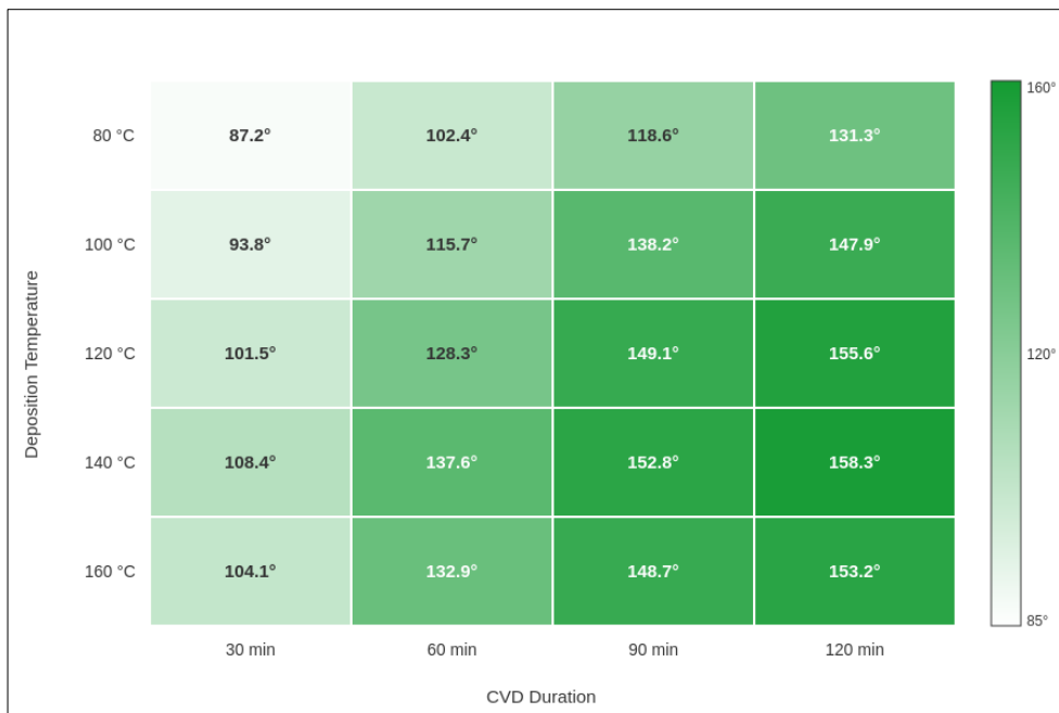
Fig 2: Heatmap showing static water contact angle (°) as a function of CVD temperature and deposition duration.
