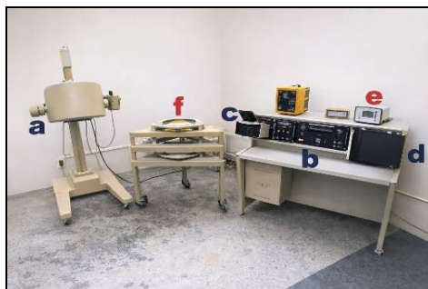
Fig 3: Shows an Anger-type scintillation camera. The detector assembly (a) consists of a collimator, scintillation crystal, and an array of photomultiplier tubes. The console features a control panel (b), an output screen for photography (c), an output screen for recording on radiographic film (d), and a device for selecting the image format (e). Additionally, various collimators (f) are available for different imaging purposes.
