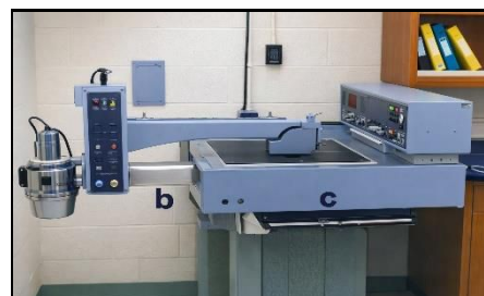
Fig 2: Displays a rectilinear scanner. The detector assembly (a) comprises a collimator, scintillation crystal, and photomultiplier tube. The rigid bar (b) links the detector to the light source, which is responsible for exposing the film inside the film holder (c).
