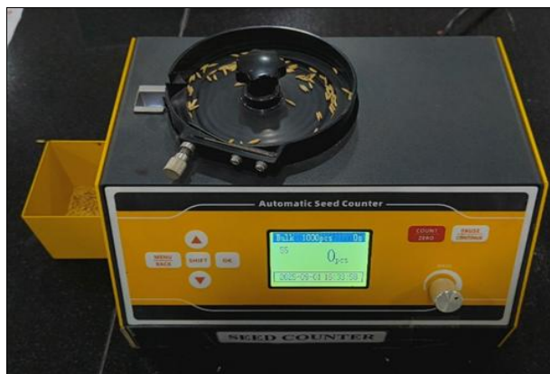
Plate 4: Measurement of 1000 paddy seeds count using digital seed counter
