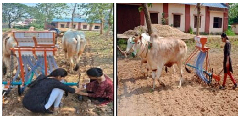
Fig 2: Field testing of seed drill
