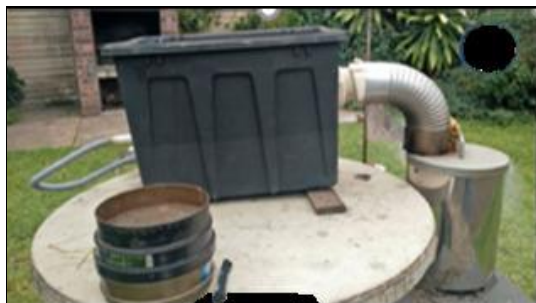
Fig 3: Apparatus designed for the preparation of smoke water (Gupta et al. , 2020) [9].
