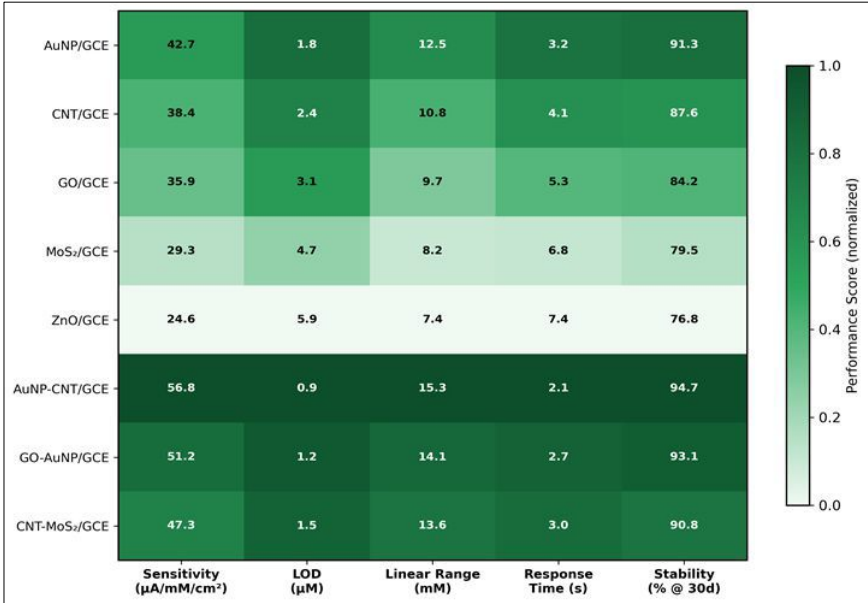
Fig 2: Heatmap visualization of normalized performance metrics for eight nanomaterial-modified electrode configurations. Darker green indicates superior performance for each metric. LOD and response time are inverse-scaled (lower values receive higher scores).
