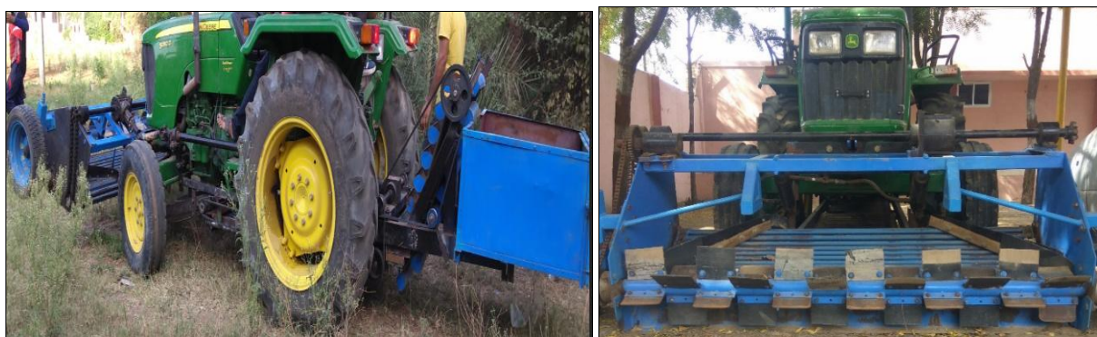
Fig 12: Integrated tractor front mounted onion harvester with inbuilt leaf de-topping unit
