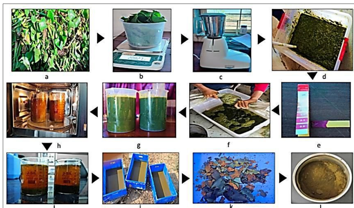
Fig 1: (a) Carefully collected apical leaves of eichhornia plant (b) Washed leaves carefully weigh (c) Cut into pieces and crushed with water in the blender (Solid to liquid ratio 1:3) (d) Add 1N, NaOH to get 8.5 pH (e) The slurry was filtered with cheesecloth and separated the liquid portion (f) the separated portion was acidified with 1.0 N HCL to up to pH 4.0 (g) the whole portion heated at 82 °C for 5 min (h) Allow to settled the mixture further supernatant was decant and the remaining matrix or LPC was carefully collected after precipitation (I) Repeated the process washed with water (K) Further, dried the precipitated LPC at 60 °C and crushed into LPC powder further stored in air tight container for proximate analysis.
