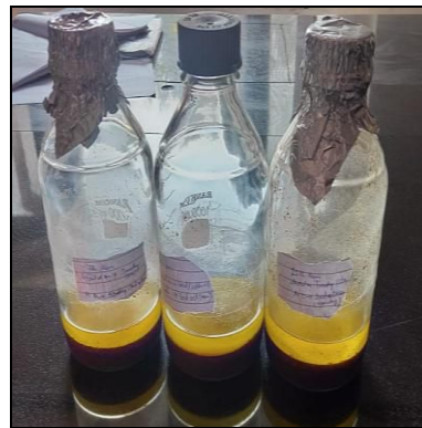
Fig 2: Maceration extraction of the silkworm pupal oil
