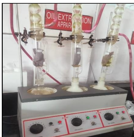
Fig 1: Soxhlet extraction of silkworm pupal oil
