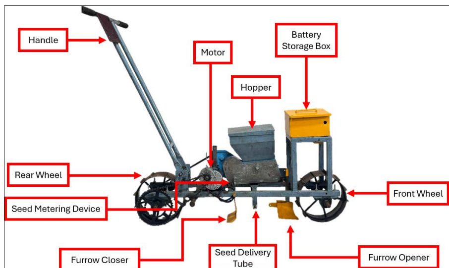
Fig 1: Design of battery-operated belt-type vegetable seed planter assembly with labeled components
