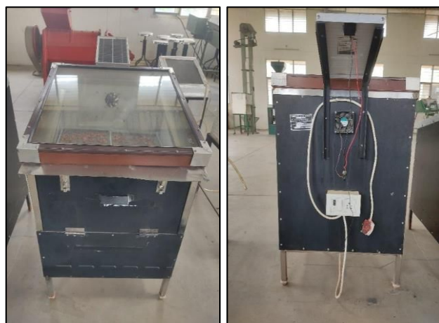
Fig. 3. Existing solar cabinet dryer
