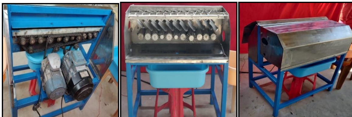
Fig 1: Assembled fish descaling machine a) Top view b) Front view c) Side view
