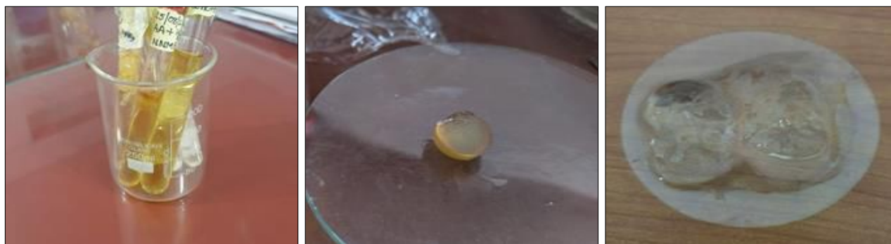
Fig 1: a) Prepared PAA gel b) Dry PAA gel c) Swollen PAA hydrogel
