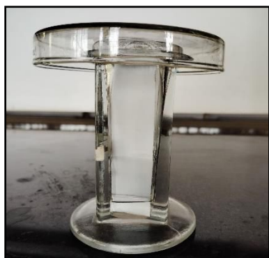
Fig 4: TLC chamber of ethyl acetate extract
