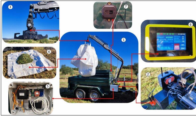
Fig 6: Components of the yield monitor. 1 Transport trailer, 2 Electronic and hydraulic system for arm control, 3 Implement with loading bolt for weighing fruit, 4 Standard big bags for loading fruit, 5 Electronic system for geo-referencing fruit big bags, weighing and sending data, 6 Wireless electronic system for logistic configuration and visualisation, 7 RTK GNSS antenna. (Olive Yield Monitor for Small Farms, ResearchGate)
