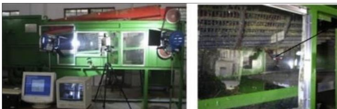
Fig 2: Grain threshing separation process under highspeed camera
