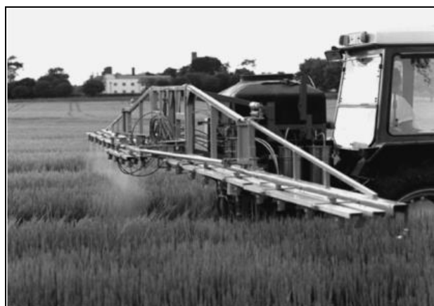
Fig 9: Stafford and Miller had created a variable rate herbicide applicator in 1993
