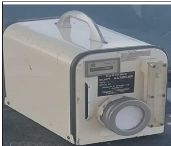
Fig 2: Senefer device for collecting suspended dust samples from atmospheric air. Source/ [11].
