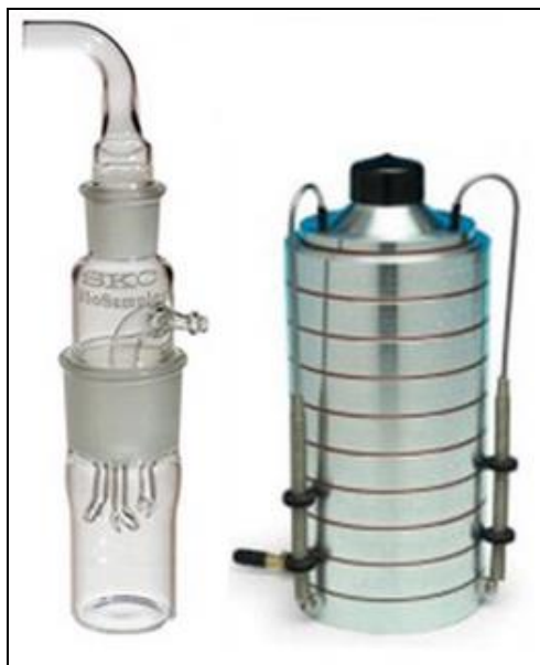
Fig 1: The cascading impact device used by scientists to collect aerosols consisting of six stages of the Andersen model [10].
