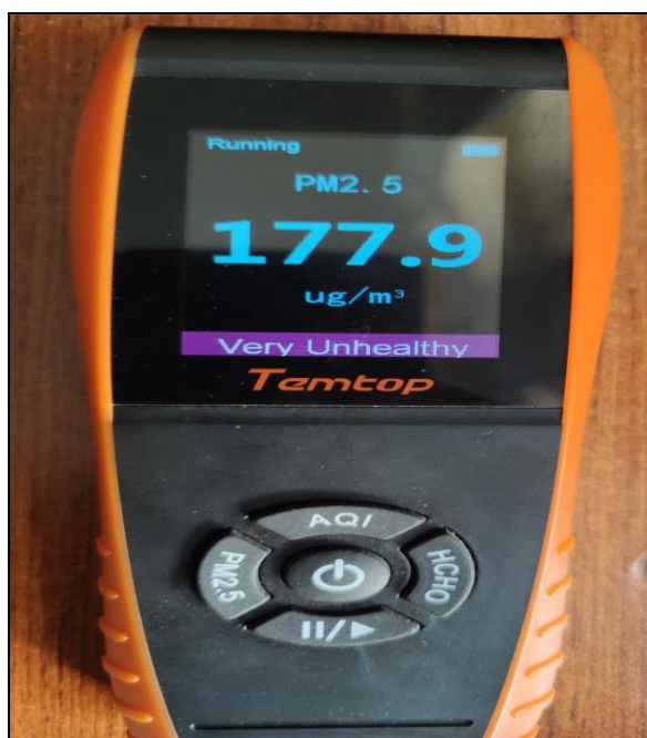
Fig 5: TEMTOP device for measuring the amount of dust suspended in the source atmospheric air/ [11] .
