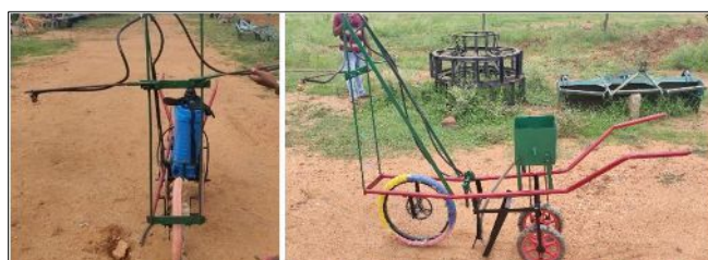
Fig 11: Multi-purpose tool carrier with seed showing and spraying mechanism
