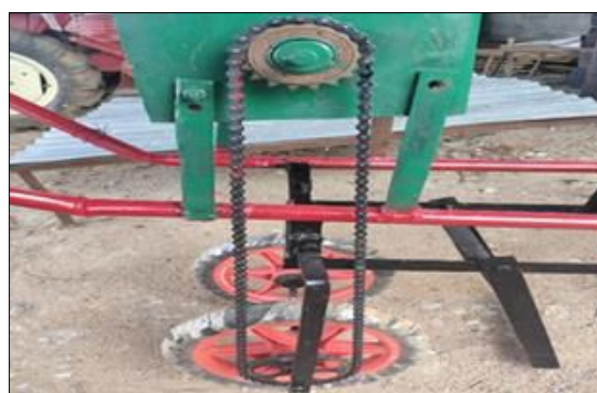
Fig 10: Chain and sprocket arrangement for seed metering mechanism
