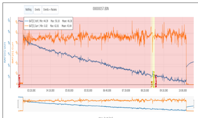
Fig 3: Battery Voltage and Current Graph (Without payload) demonstrates the battery consumption trend.
