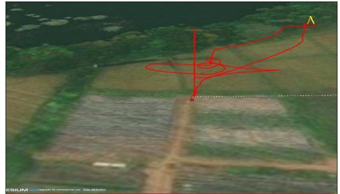
Fig 1: 3D Flight Path Trajectory (Altitude & Range) illustrates the UAV's flight path and altitude consistency.
