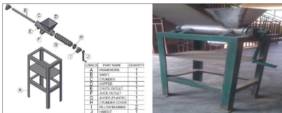
Fig 5: Isometric and photographic view of the manual fruit juice extraction machine
