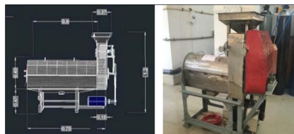
Fig 12: Orthographic and photographic image of the fabricated Kendu pulper
