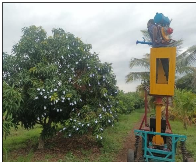
Fig 3: Testing of developed tractor operated raising platform for spraying on mango trees
