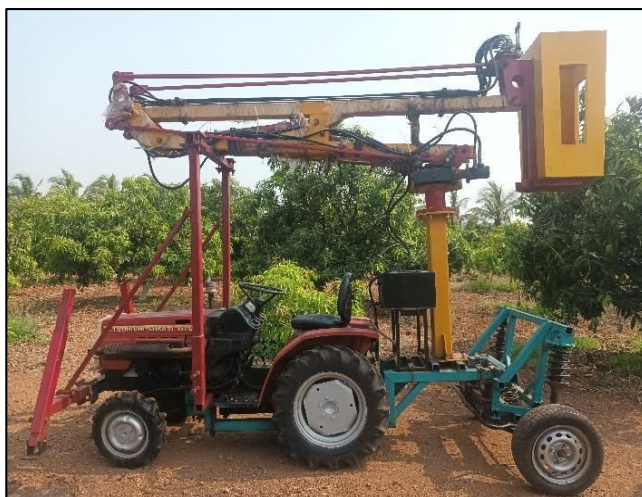
Fig 1: Developed small tractor operated raising platform (elevator)
