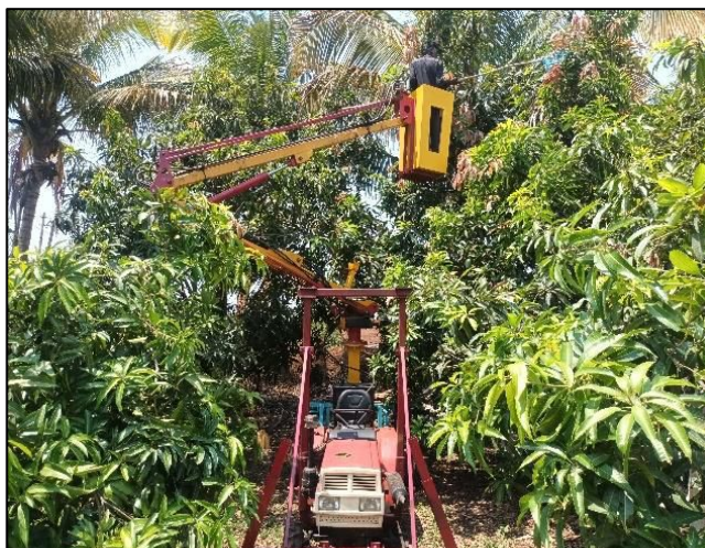
Fig 3: Testing of developed small tractor operated raising platform for harvesting of mango
