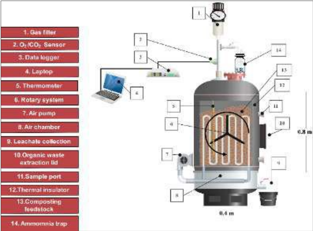
Fig 1: The schematic diagram of aerobic composting reactor
