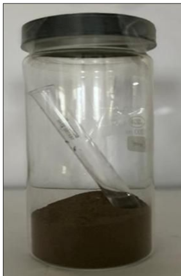
Fig 6: Experimental setup for determination of biodegradability of prepared bioplastic
