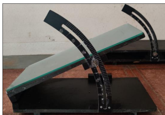
Fig 6: Apparatus for measuring the coefficient of static friction
