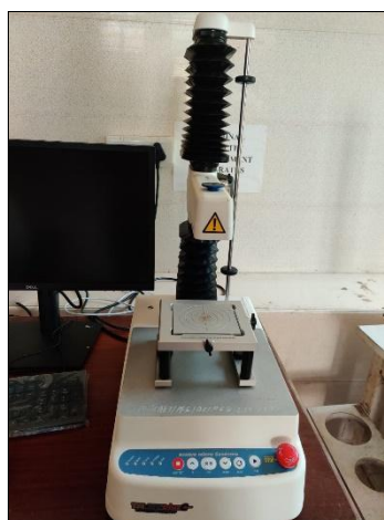
Fig 5: Texture analyzer used for measuring compressive strength
